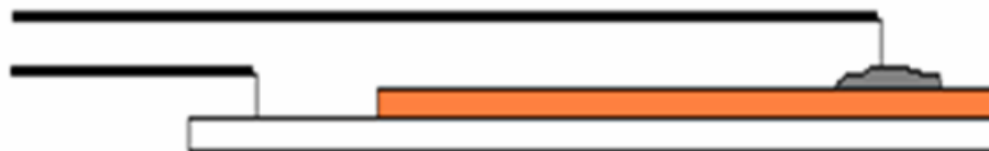
Figure 2- Electric connections on the thin film, first method
